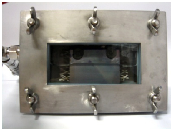
Fig. 2. Image of photocatalytic water-splitting reactor.
